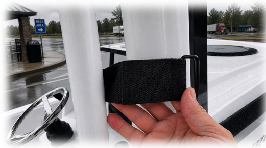
Figure 6 — Transport strap installed around the windshield support post.
